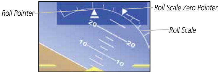
Attitude Indicator with a Ground Pointer Configuration in a Left Turn
