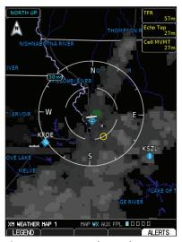
Figure 4-43 XM Weather - Echo Tops
