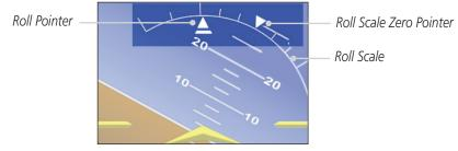
Figure 2-15 Attitude Indicator with Ground Pointer Configuration in a Left Turn
