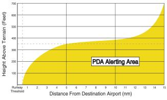
Figure 4-19 PDA Alerting Threshold
