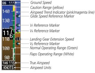
Figure 2-7 Airspeed Tape
