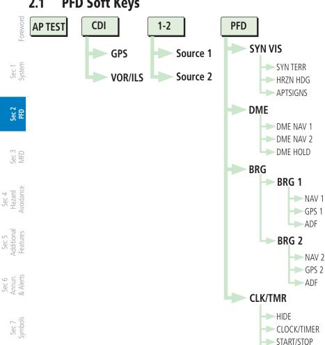
Figure 2-3 PFD Soft Key Diagram
