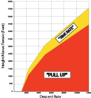
Figure 4-18 Excessive Descent Rate Alert Criteria
