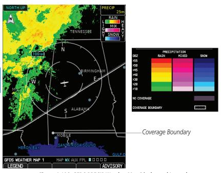
Figure 4-106 GFDS PRECIP Weather Map Display and Legend
