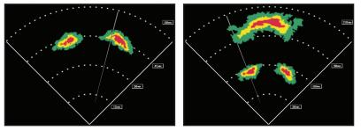
Figure 4-79 The "Blind Alley" Horizontal Scan
