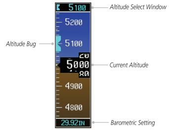
Figure 1-19 Pressing PFD Knob Sets Altitude Select to Current Altitude
