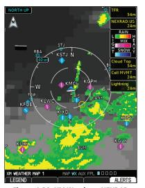
Figure 4-38 XM Weather - NEXRAD
