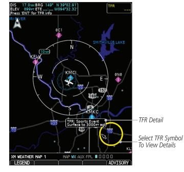
Figure 4-59 XM Weather - TFRs
