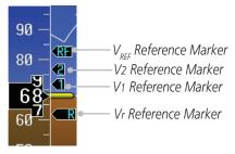
Figure 2-12 Alternate Reference Speeds
