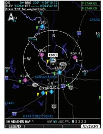
Figure 4-49 XM Weather - Graphic METARs
