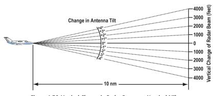
Figure 4-76 Vertical Change in Radar Beam per Nautical Mile
