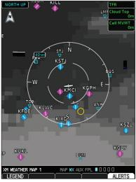
Figure 4-44 XM Weather - Cloud Tops
