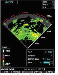
Figure 4-90 Horizontal Scan without WATCH™ Figure 4-91 Horizontal Scan with WATCH™
