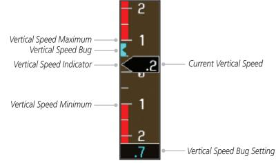
Figure 1-21 Vertical Speed Warning Indication
