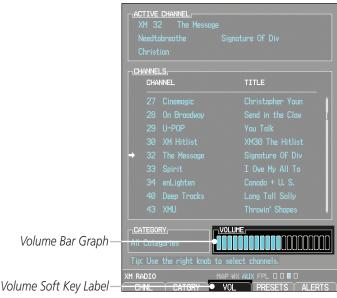
Figure 5-26 XM Radio Volume Setting
