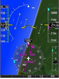
Figure 2-20 Extreme Roll Indication with Display Declutter
