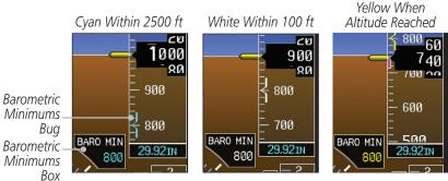
Figure 2-24 Barometric MDA/DH - Alerting Visual Annunciations
