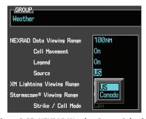
Figure 3-27 NEXRAD Weather Source Selection
