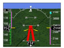
Figure 2-18 Extreme Pitch Indication - Nose Down
