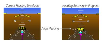
Figure 1-9 AHRS Heading Indications
