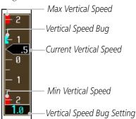
Figure 2-26 Vertical Speed Tape and Window
