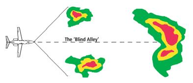
Figure 4-78 The "Blind Alley" Overhead View
