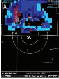
Figure 4-66 XM Weather - Icing and SLD
