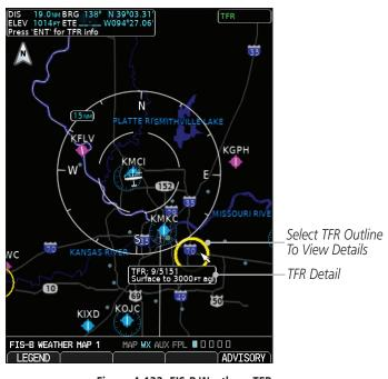
Figure 4-132 FIS-B Weather - TFRs
