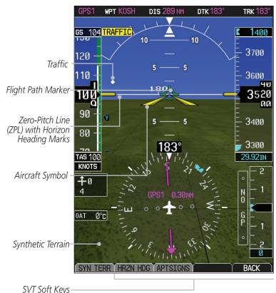
Figure 5-43 SVT on Primary Flight Display
