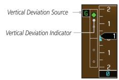
Figure 2-33 Vertical Deviation Indicator (ILS Source)
