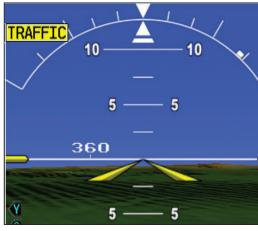
Figure 5-41 Pitch Scale with SVT Enabled
