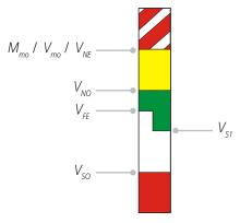
Figure 2-9 Typical Airspeed Tape Markings
