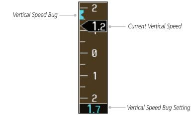
Figure 1-20 Pressing V/S Knob Sets Vertical Speed Bug to Current Vertical Speed
