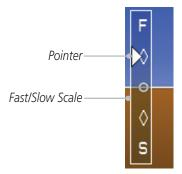
Figure 2-49 Fast/Slow Scale and Pointer
