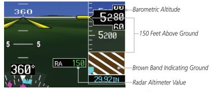
Figure 2-45 Radar Altimeter Display - 150 ft RA Altitude
