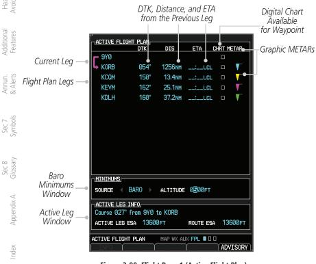
Figure 3-90 Flight Page 1 (Active Flight Plan)
