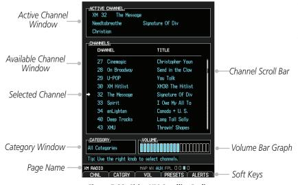
Figure 5-22 Sirius XM Satellite Radio
