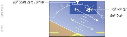
Figure 2-16 Attitude Indicator with Sky Pointer Configuration in Left Turn
