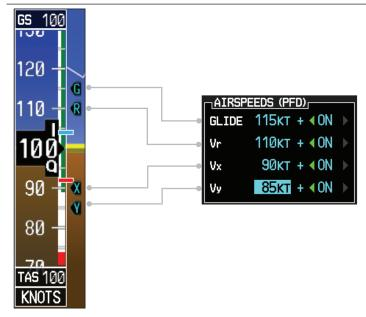
Figure 3-40 Airspeed References shown on PFD when activated
