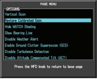
Figure 4-87 Restore Calibrated Gain
