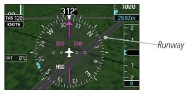
Figure 5-46 Depiction of Runway with a Loaded Flight plan
