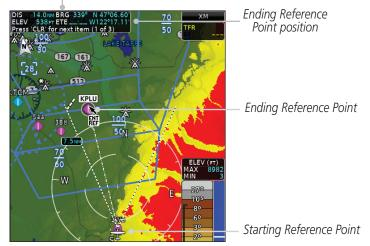
Figure 3-10 Bearing/Distance Measurement
