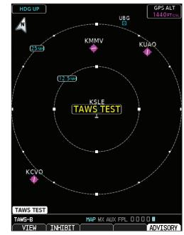
Figure 4-15 TAWS Test Display and PFD Annunciation
