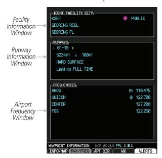
Figure 3-100 Flight Plan Waypoint Info Detail
