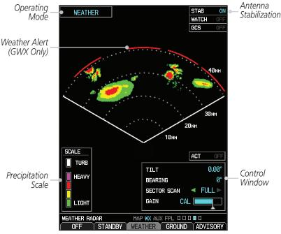
Figure 4-80 Horizontal Scan Display
