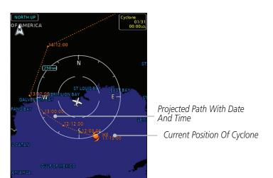
Figure 4-64 XM Weather - Cyclone
