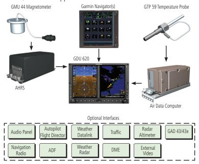
Figure 1-1 G500/G600 System (LRU Configuration)
