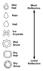
Figure 4-73 Precipitation Type and Reflectivity
