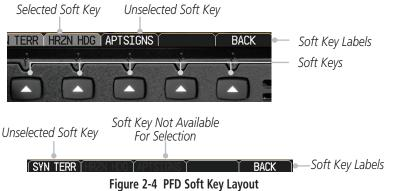
When a soft key is selected, its color changes to black text on gray background and remains this way until it is turned off, at which time it reverts to white text on black background. When a soft key function is disabled, the soft key label is subdued (dimmed).
