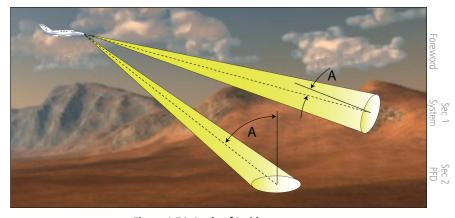
Figure 4-74 Angle of Incidence
