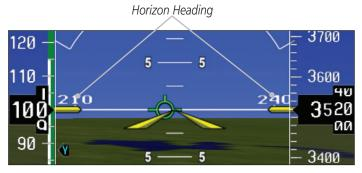
Figure 5-44 Horizon Heading
