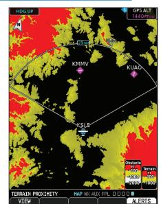
Figure 4-7 Terrain Page with Aviation Data Displayed and 120° Arc View
