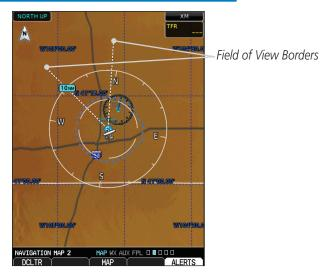
Figure 3-22 Navigation Map Field of View on the MFD
