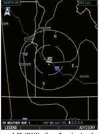
Figure 4-65 XM Weather - Freezing Levels
