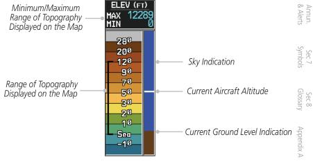
Figure 3-18 Navigation Map Topo Scale
