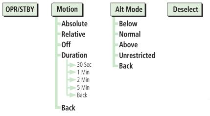
Figure 4-31 ADS-B Traffic Page Functional Diagram
