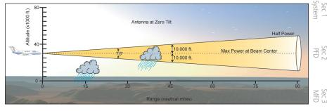
Figure 4-71 Radar Beam from 12 inch Antenna
