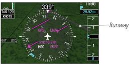
Figure 5-47 Depiction of Runway Not in Loaded Flight plan
