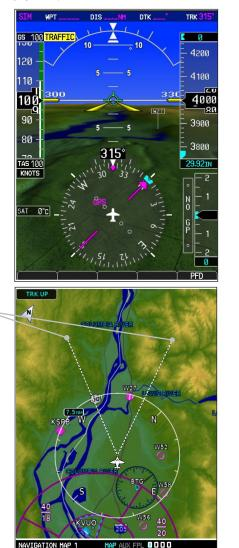
Figure 5-51 MFD and PFD Field of View Comparison
