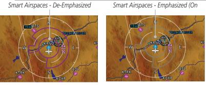
Figure 3-31 Display of Smart Airspaces (Airspace Borders Grayed When Emphasized)
