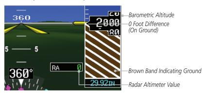
Figure 2-46 Radar Altimeter Display - 0 ft RA Altitude
