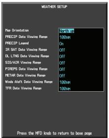
Figure 4-98 Weather Data Link Setup Menu Options
