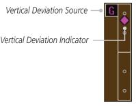
Figure 2-34 Vertical Deviation Indicator (GPS Source)
