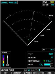
Figure 4-68 Ground Mapping Display
