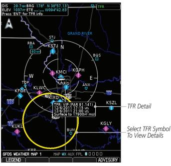
Figure 4-118 GFDS Weather - TFRs
