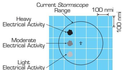
Figure 4-1. Airspace Diagram
