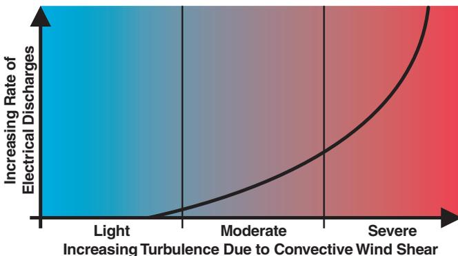
Figure 2-2. Discharge Rate a Function of Wind Shear
