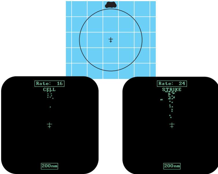
Figure 4-11. Discharge Points Off the Aircraft's Nose
