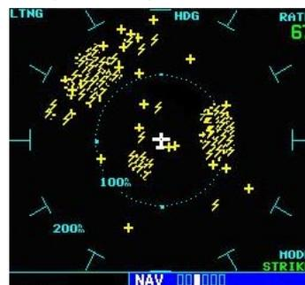
For lightning display interpretation, study the examples in the WX-500 Pilot's Guide that are designed to help you relate the cell or strike patterns shown on the display to the size and location of thunderstorms that may be near your aircraft.
