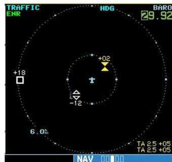
The Barometric Pressure field is located in the upper right-hand corner of the Traffic Page.
