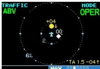
Operating Mode is confirmed by the display of "OPER" in the upper right-hand corner of the Traffic Page.
