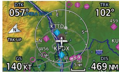
Figure 8-26 Display of Smart Airspaces (Airspace Borders Grayed)
