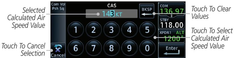
Figure 14-43 Select Calculated Air Speed Value
