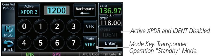
Figure 2-7 Transponder Mode "Standby" Indication
