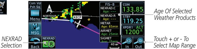
**Figure 11-72 FIS-B Weather Page (NEXRAD Key Shown)**
