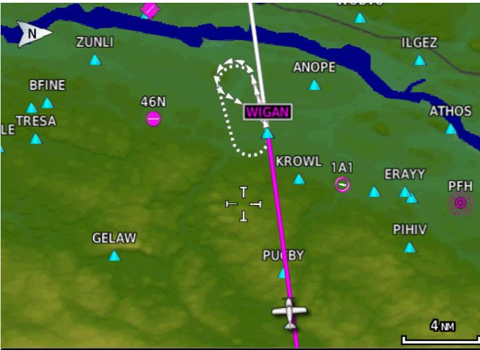
Figure 8-57 Active Flight Plan Leg Prior to Holding Pattern
