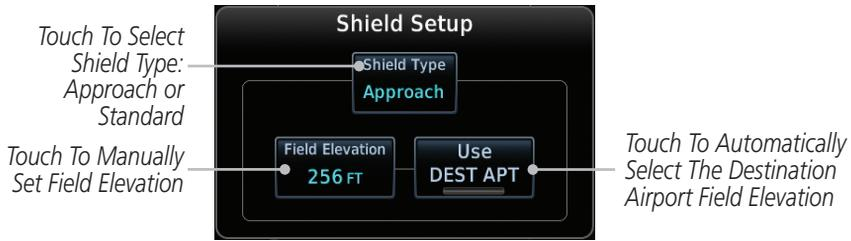
**Figure 9-28 TCAD 9900B Shield Setup for Approach**
