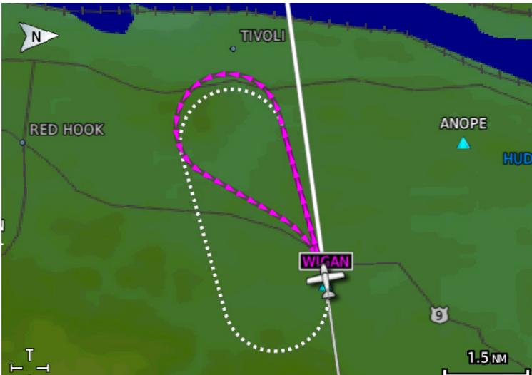
**Figure 8-49 Holding Pattern Entry**
