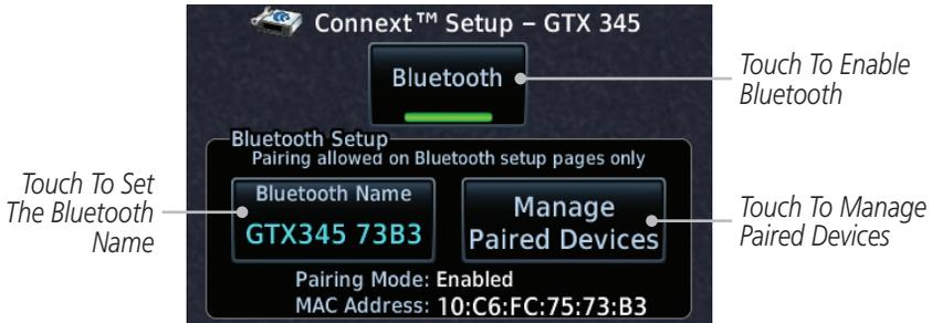
**Figure 15-56 Connex Setup for GTX 345**
