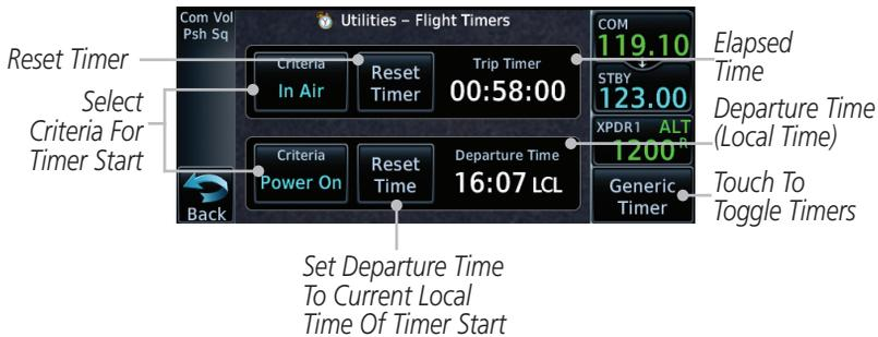
Figure 14-12 Utility Flight Timers Page (Trip/DEP Timers)
