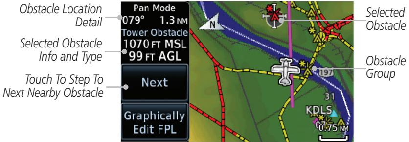
Figure 8-23 Point Obstacle Detail
