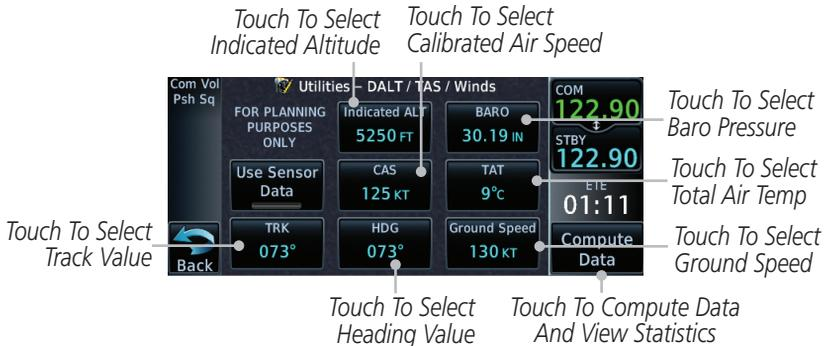
**Figure 14-39 Utility DALT/TAS/Winds Page Using Manually Entered Data**
