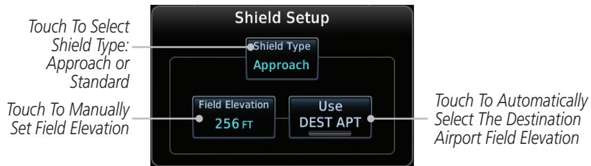
Figure 9-34 TCAD 9900BX Shield Setup for Approach
