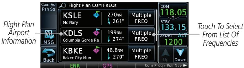
Figure 3-14 Flight Plan Frequency List
