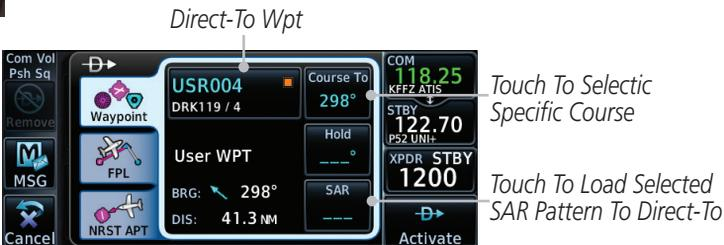
Figure 5-14 Create SAR Pattern at Direct-To Waypoint
