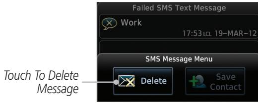
Figure 13-27 Delete a Failed SMS Text Message
