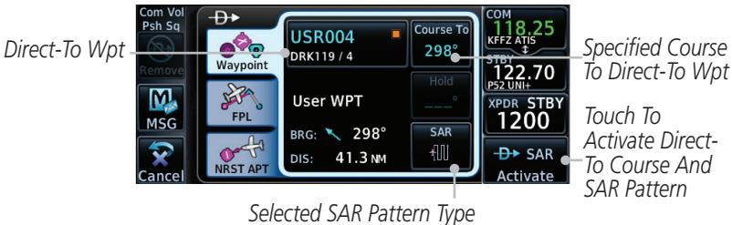
**Figure 5-17 Direct-To Page with SAR Pattern Selected**
