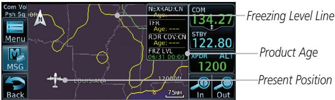
Figure 11-25 Freezing Level
