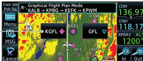
Figure 8-43 Select the Desired Waypoint From Multiple Waypoints
