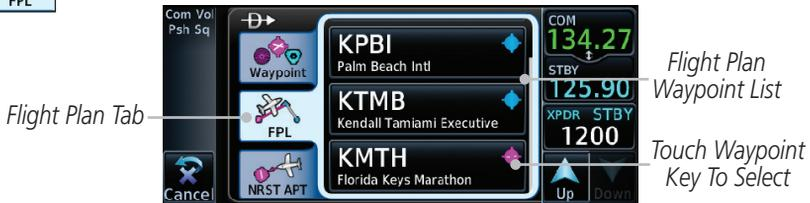
Figure 5-4 Direct-To Flight Plan Leg Selection
