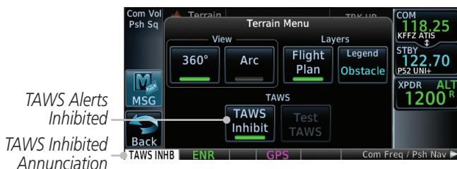
Figure 10-14 TAWS-B Alerting Disabled (TAWS Inhibited) Annunciation
