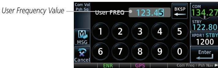
**Figure 3-22 Select a Frequency Value for the New User Frequency**
