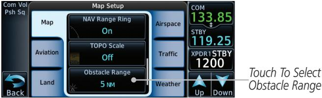
Figure 8-20 Map Setup For Obstacle Range
