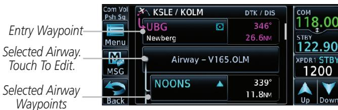
Figure 4-24 Airway Waypoints in the Flight Plan
