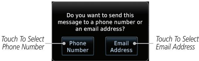
**Figure 13-24 Select Destination for the SMS Text Message**
