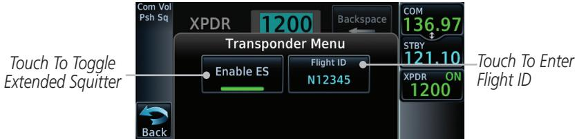
Figure 2-16 Transponder Menu With Extended Squitter Capability
