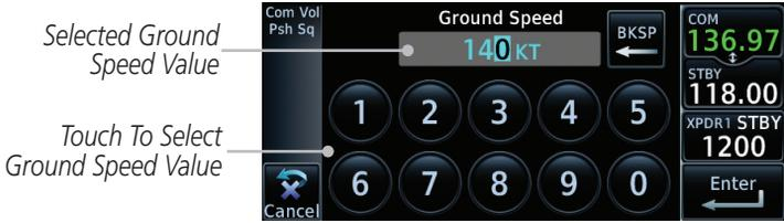
Figure 14-32 Selecting Ground Speed
