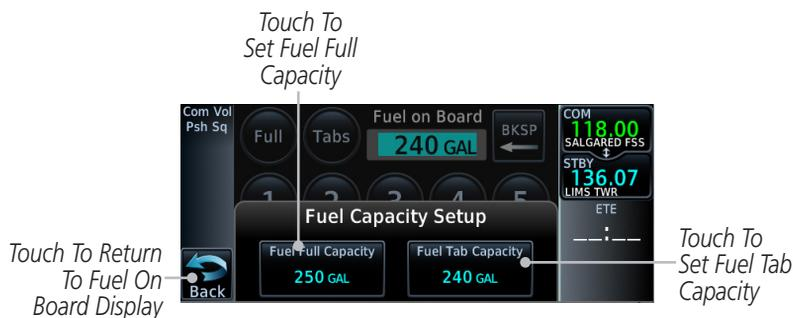
Figure 1-14 Fuel Capacity Setup Page
