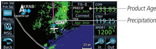
Figure 11-62 Connex Precipitation Data
