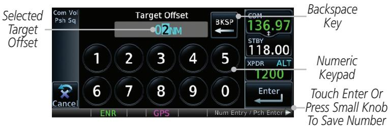
Figure 14-8 Select VCALC Target Offset
