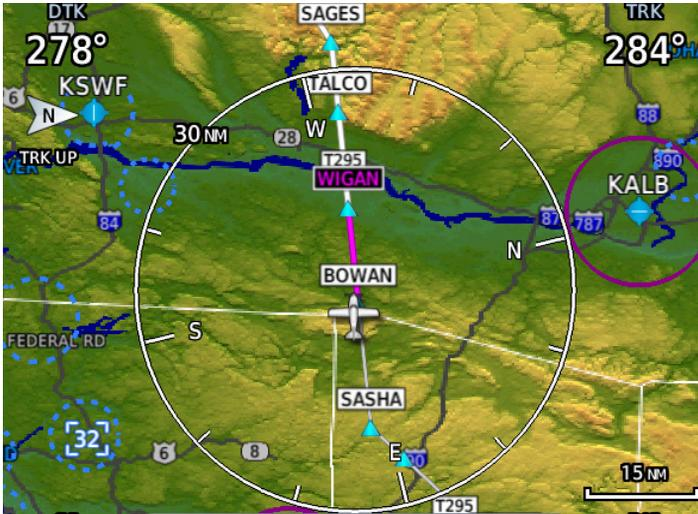
Figure 8-54 Past, Active, and Future Flight Plan Segments
