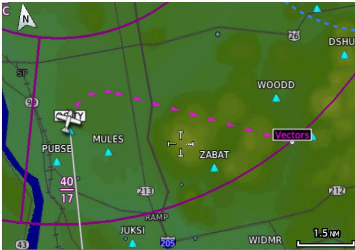
Figure 8-55 Active Heading Leg (Vectors)
