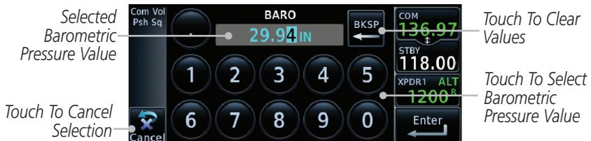
**Figure 14-42 Select Barometric Pressure Value**
