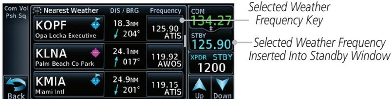
Figure 12-25 Nearest Weather Station Selected Frequency
