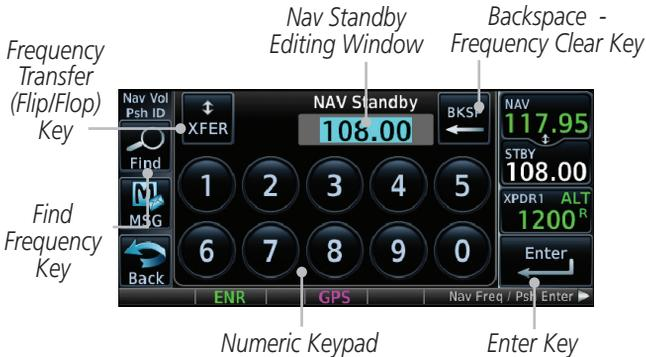
**Figure 3-6 Nav Standby Frequency Numeric Keypad**
