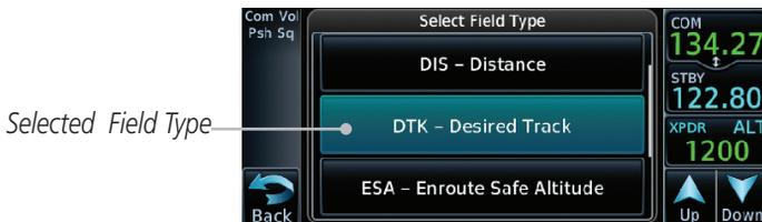
Figure 4-48 Flight Plan Data Fields List
