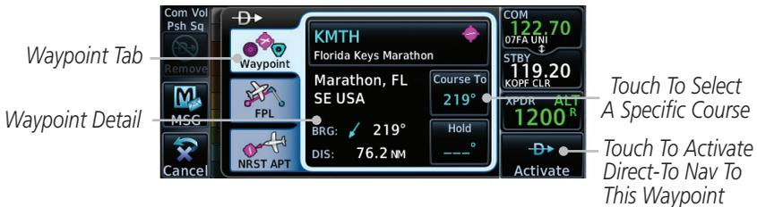
Figure 5-5 Selected Direct-To Flight Plan Leg
