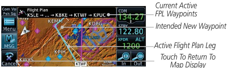
Figure 8-40 Drag Selected Leg of Flight Plan to New Waypoint
