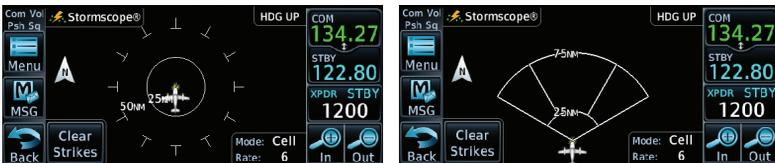
Figure 11-48 StormScope 360° and Arc Display Views
