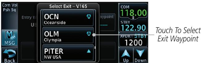
**Figure 4-21** Select an Exit Waypoint for the Airway
