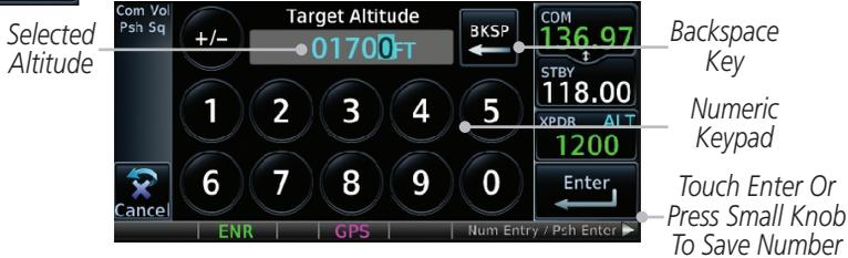
Figure 14-6 Select VCalc Target Altitude
