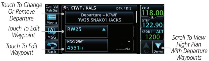
**Figure 6-7 Flight Plan View of the Selected Departure**
