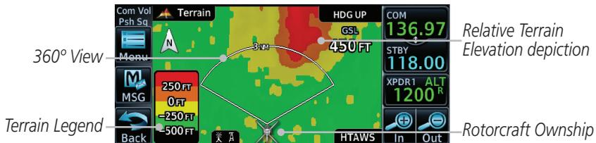
Figure 10-20 Terrain Page with HTAWS - 120° View
