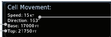
Figure 11-19 Cell Movement Detail
