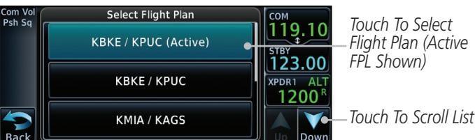
**Figure 14-23 Select Flight Plan**
