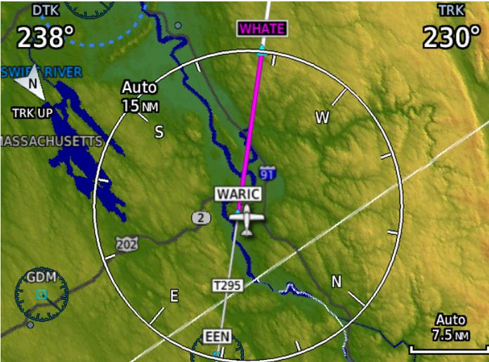
Figure 8-56 Active Flight Plan Leg
