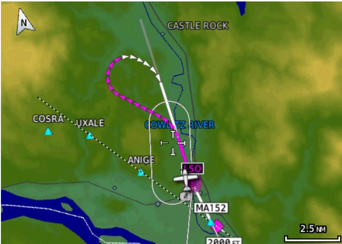
**Figure 8-53 Active Procedure Turn**
