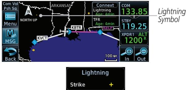
Figure 11-63 Connex Data Link Lightning and Legend
