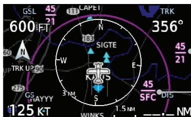
**Figure 8-25 Display of Airspace Labels**
