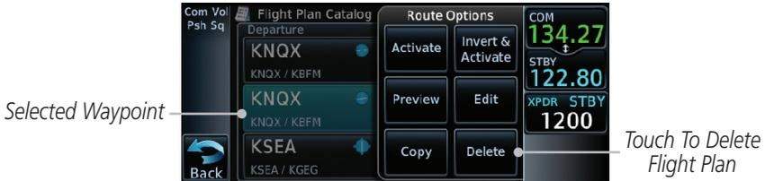
Figure 4-57 Select Flight Plan from the Catalog to Delete
