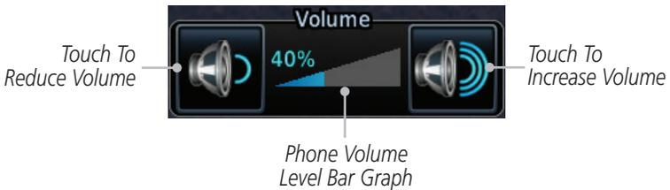
**Figure 13-20 Select Soft Keys for Phone Volume Adjustment**
