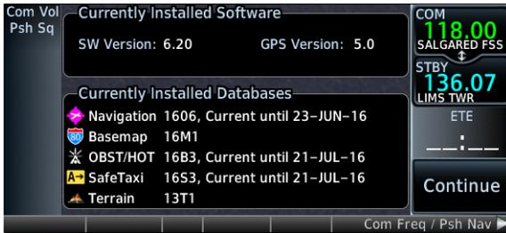
**Figure 18-5** Currently Installed Software/Databases
