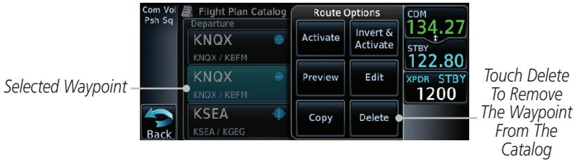
Figure 4-59 Select a Flight Plan from the Catalog
