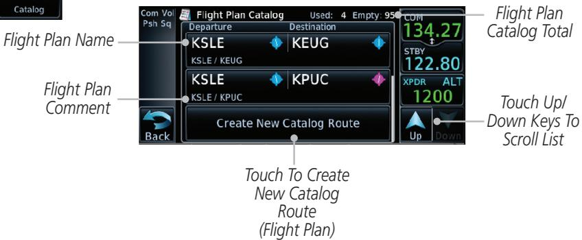
Figure 4-49 Flight Plan Catalog
