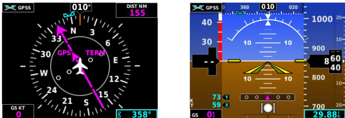
When GPSS is selected on the G5, GPSS turn commands are converted into a heading error signal to the autopilot. When the autopilot is operated in HDG mode, the autopilot will fly the turn commands from the GPS navigator. If the GPSS data is invalid (for example, if there is no active GPS leg) or the selected navigation source on the G5 ADI and HSI is not GPS, the annunciated GPSS text will be yellow and a zero turn command will be sent to the autopilot.
