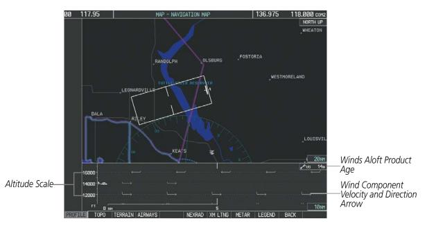
Figure 6-34 Navigation Map Page with Winds Aloft Weather Product on Profile View
