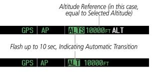
Figure 7-6 Automatic Mode Transitions During Altitude Capture
