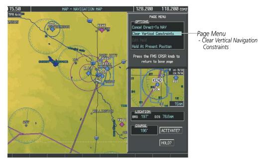
Figure 5-55 Direct-to Window - Clearing Vertical Constraints
