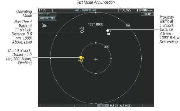
Figure 6-164 System Test in Progress with Test Pattern
