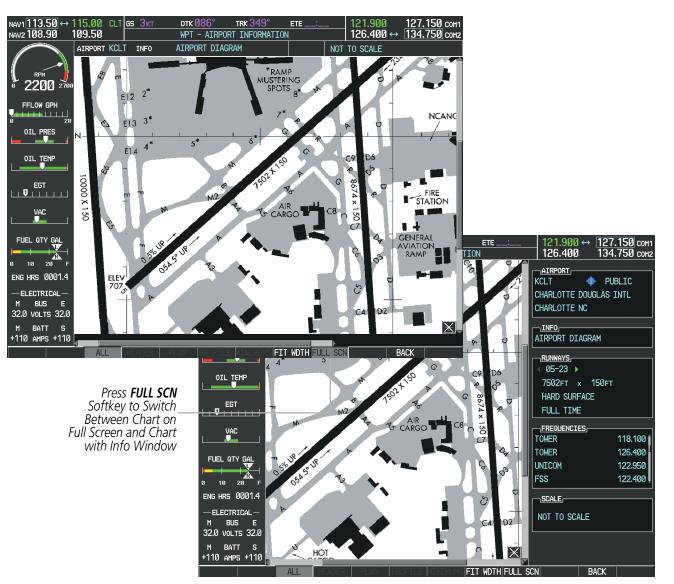
Pressing the **FULL SCN** Softkey alternates between removing and replacing the data window to the right.
