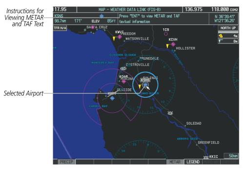
Figure 6-108 METAR Flags on the Weather Data Link Page
