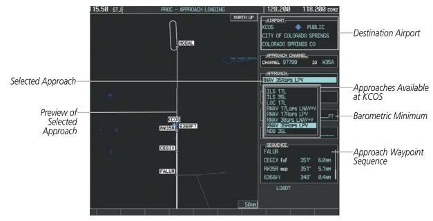
Figure 5-74 Approach Loading Page - Selecting the Approach
