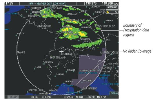
Figure 6-69 Precipitation Data on the Weather Data Link (CNXT) Page
