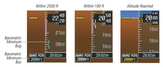
Figure 2-38 Barometric MDA/DH Alerting Visual Annunciations
