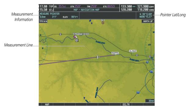
Figure 5-13 Navigation Map - Measuring Bearing and Distance
