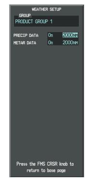
Figure 6-102 Weather Data Link (FIS-B) Page Setup Menu
