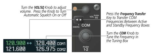
Figure 4-5 COM Frequency Tuning
