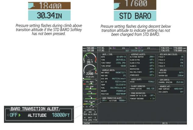
Figure 2-10 Baro Transition Alert (AUX - System Setup Page)
