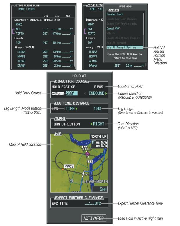
Figure 5-90 Creating a User Defined Holding Pattern at the Aircraft Present Position
