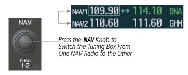
Figure 4-20 Switching NAV Tuning Boxes
