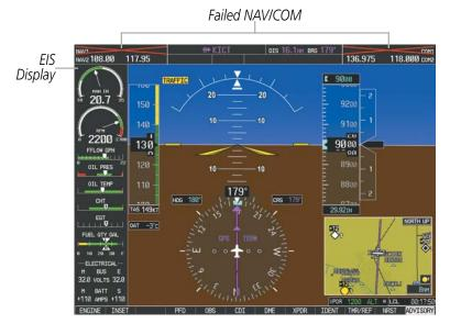
Figure 3-2 Primary Flight Display (182T Reversionary Mode)
