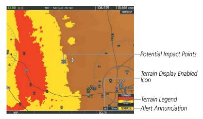
Figure 6-146 Navigation Map Page (After TAWS-B Pop-up Alert Acknowledgment)
