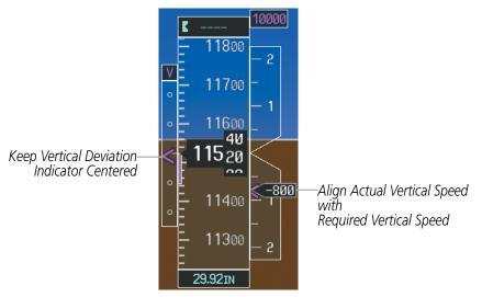
Figure 5-138 VDI & RVSI Showing Correctly Established Descent
