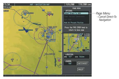
Figure 5-54 Direct-to Window - Cancelling Direct-to Navigation
