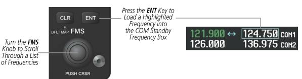
Figure 4-9 Frequency Auto-Tuning from the MFD
