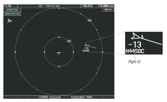
Figure 6-166 Traffic Map Page with Flight ID Enabled
