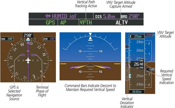
Figure 7-12 Vertical Path Tracking Mode
