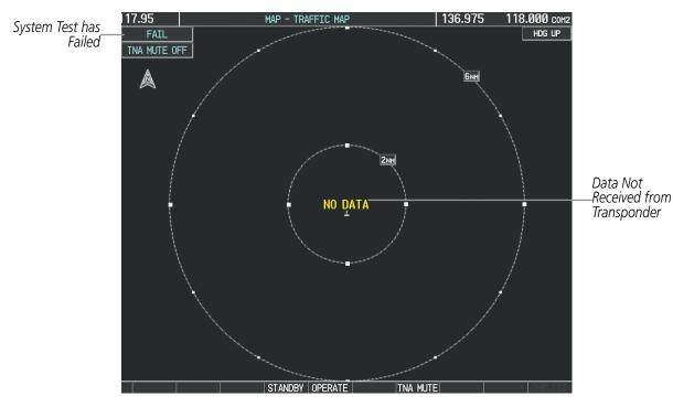
Figure 6-160 TIS Power-up Test Failure
