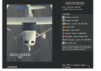
Figure 1-8 MFD Power-Up Screen (172R shown)
