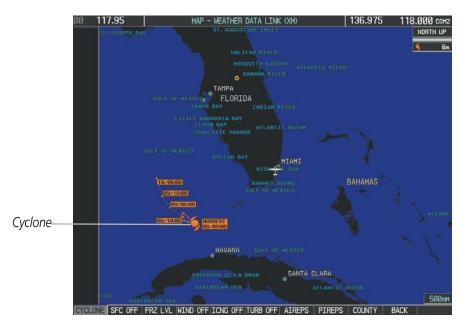
Figure 6-40 Cyclone Data Selected for Display
