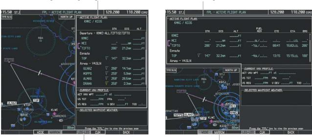
WIDE Softkey, NARROW Softkey, LEG-LEG Softkey, CUM Softkey Figure 5-87 Active Flight Plan - Wide vs. Narrow View
