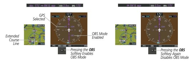
Figure 2-26 Omni-bearing Selector (OBS) Mode
