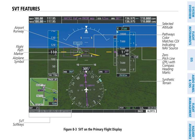
**NOTE:** Pathways and terrain features are not a substitute for standard course and altitude deviation information provided by the altimeter, CDI, and VDI.
