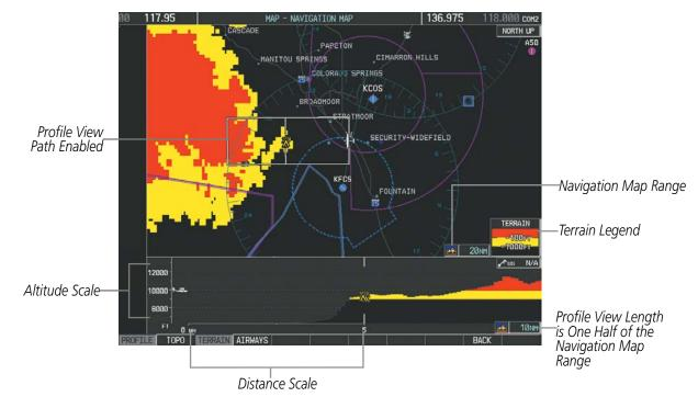
Figure 6-123 Profile View on Navigation Map with Terrain Display Enabled
