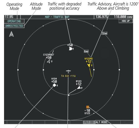
Non-threat traffic, Aircraft is 5000' Above, Descending, Undetermined Direction "Non-Bearing" Traffic, Distance is 8.0 nm, 1100" Above and Descending Non-Aircraft Ground Traffic, 1000' Below
