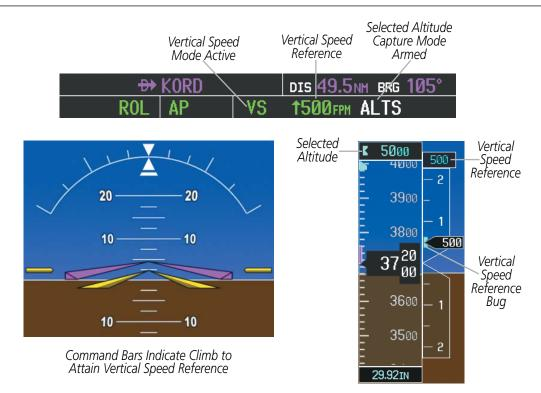
Figure 7-8 Vertical Speed Mode
