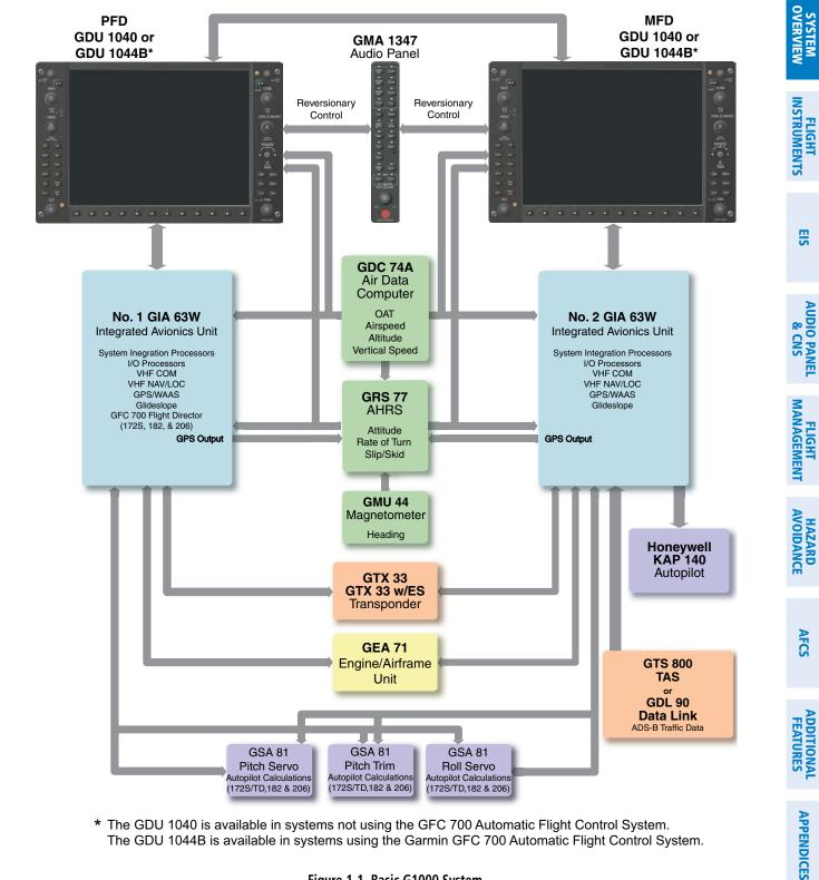
\* The GDU 1040 is available in systems not using the GFC 700 Automatic Flight Control System. The GDU 1044B is available in systems using the Garmin GFC 700 Automatic Flight Control System.
