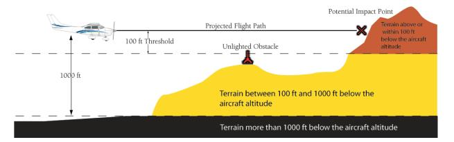
Figure 6-127 Terrain Altitude/Color Correlation for Terrain-SVS
