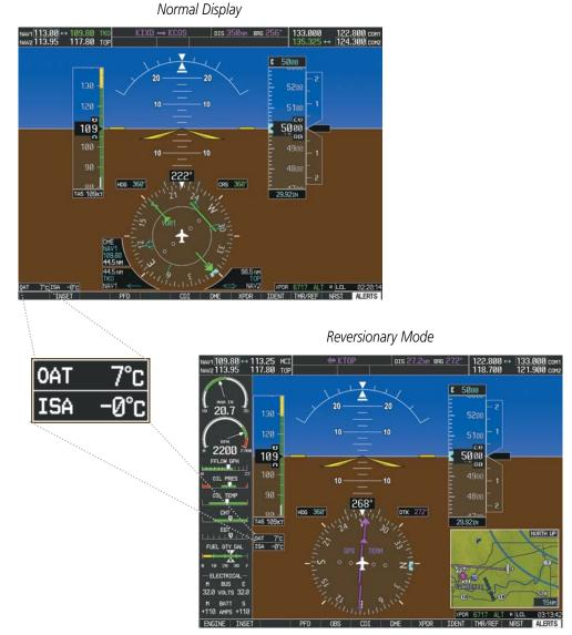
Figure 2-28 Outside Air Temperature
