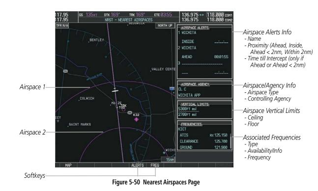
Airspace alerts and associated frequencies are shown in scrollable lists on the Nearest Airspaces Page. The ALERTS and FREQ softkeys place the cursor in the respective list. The FREQ Softkey is enabled only if one or more frequencies exist for a selected airspace.
