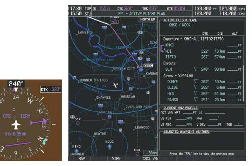
Figure 5-110 Assigned Heading of 240°
