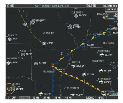
Figure 6-28 Current Surface Analysis Data
