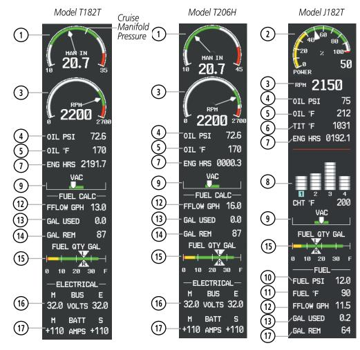
Figure 3-11 System Display (Turbocharged Aircraft)
