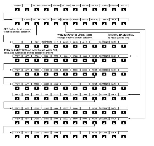
Figure 6-3 Weather Data Link (XM) Weather Product Softkeys
