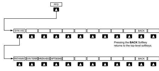
Pressing the **BACK** Softkey returns to the previous level of softkeys.
