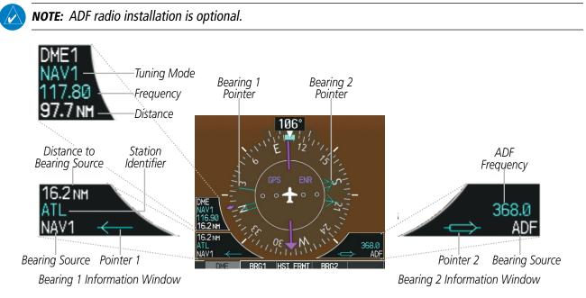
Figure 2-18 HSI with Bearing and Distance Information
