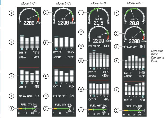
Figure 3-8 Lean Display (Normally-Aspirated Aircraft)
