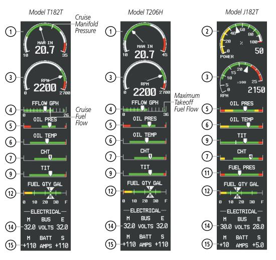
Figure 3-6 Engine Display (Turbocharged Aircraft)
