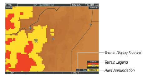
Figure 6-134 Navigation Map Page (After Terrain-SVS Pop-up Alert Acknowledgment)
