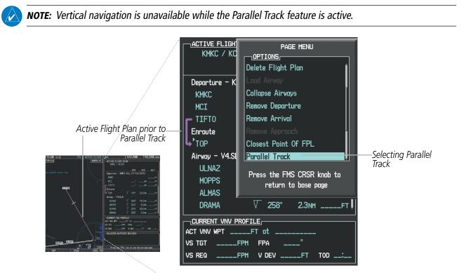
Figure 5-79 Active Flight Plan Window - Selecting Parallel Track
