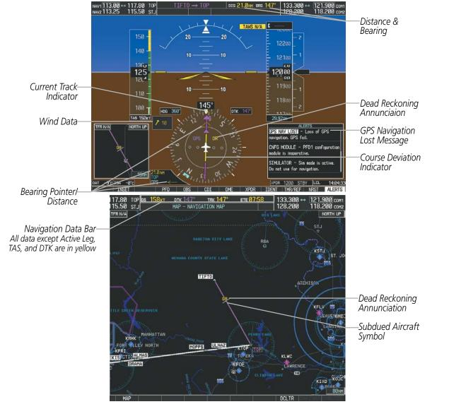
Figure 5-151 Dead Reckoning Mode - GPS Derived Data Shown in Yellow
