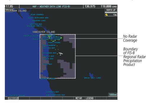
Figure 6-105 Regional Radar Precipitation Data on the Weather Data Link (FIS-B) Page)
