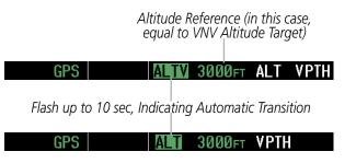
Figure 7-14 Automatic Mode Transitions During Altitude Capture
