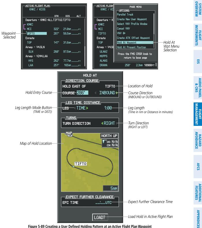
Figure 5-89 Creating a User Defined Holding Pattern at an Active Flight Plan Waypoint
