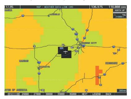
Figure 6-44 Turbulence Data at 21,000 Feet
