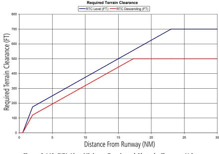
Figure 6-148 FLTA Alert Minimum Terrain and Obstacle Clearance Values
