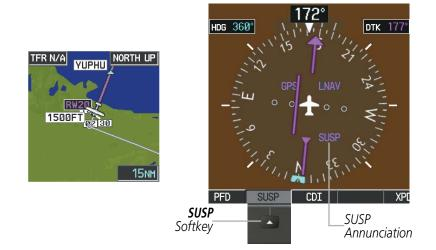
Figure 2-27 Suspending Automatic Waypoint Sequencing
