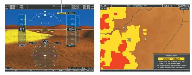
Alerts are issued when flight conditions meet parameters that are set within Terrain-SVS software algorithms. Terrain-SVS alerts typically employ a CAUTION or a WARNING alert severity level, or both. When an alert is issued, visual annunciations are displayed and voice alerts are simultaneously issued. Table 6-18 shows
