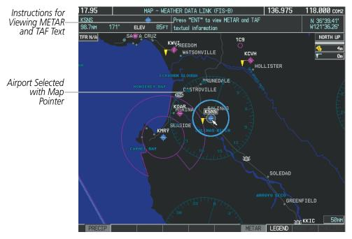
Figure 6-103 Panning on the Weather Data Link (FIS-B) Page)
