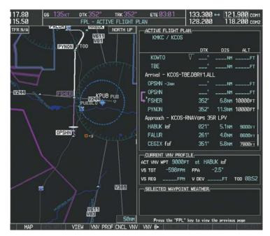
Figure 5-141 Tracking the OPSHN to FSHER Leg
