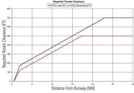
Figure 6-135 FLTA Alert Minimum Terrain and Obstacle Clearance Values
