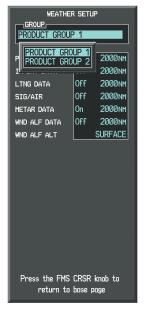
Figure 6-61 Weather Data Link (CNXT) Page Setup Menu
