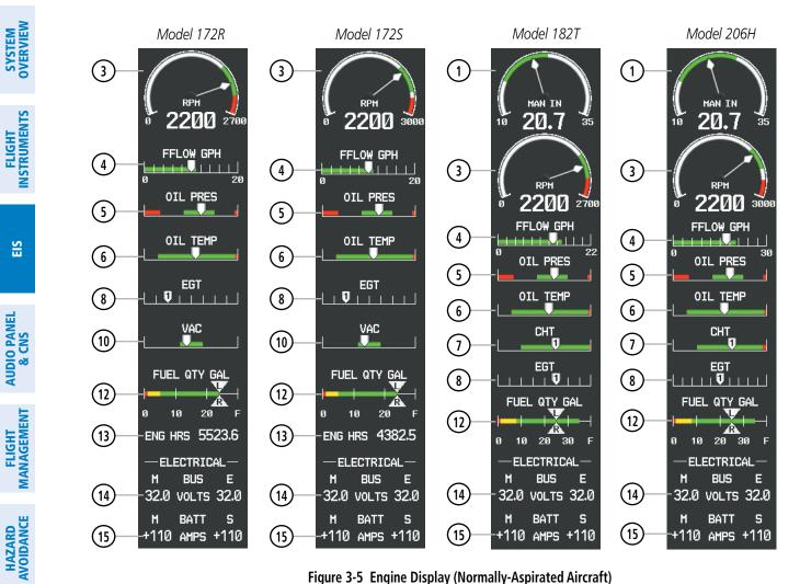
Figure 3-5 Engine Display (Normally-Aspirated Aircraft)
