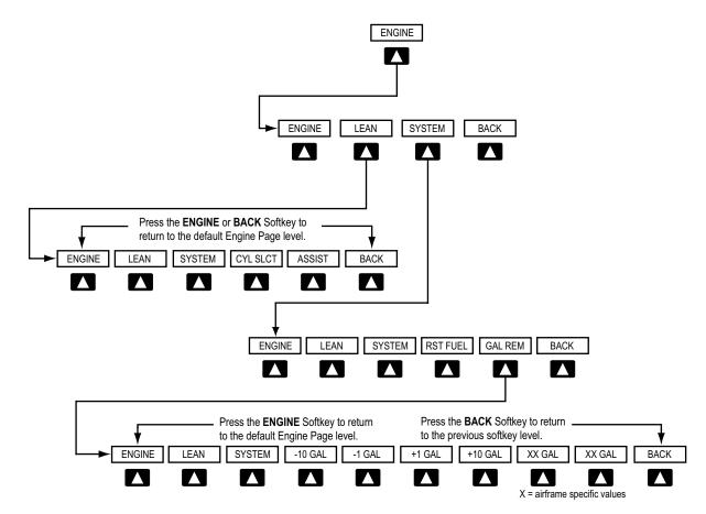
Figure 3-3 Engine Softkey Flowchart (Models 172R, 172S, 182T, 206H, T182T, and T206H)
