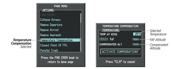
Figure 5-100 Temperature Compensation
