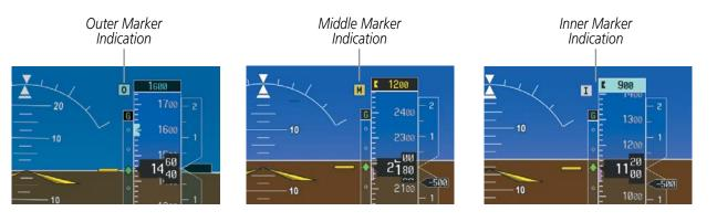
Figure 4-27 Marker Beacon Annunciations on the PFD
