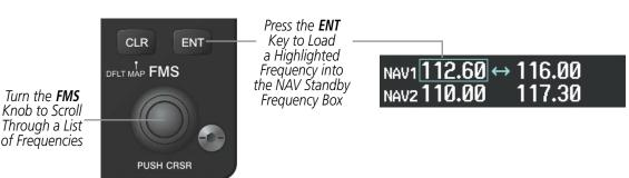
Figure 4-23 NAV Frequency Auto-Tuning from the MFD
