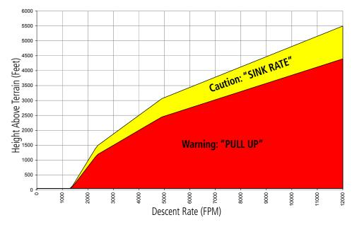
Figure 6-147 Excessive Descent Rate Alert Criteria
