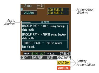
Figure 2-32 System Alerting
