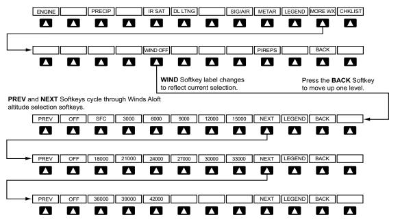
Figure 6-59 Weather Data Link (CNXT) Page (MFD)
