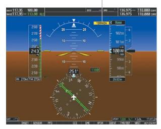
Figure 6-144 TAWS-B PFD Alert Annunciation
