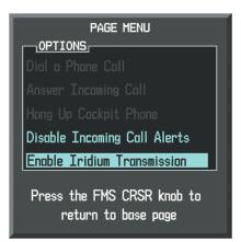
Figure 8-77 Enable Iridium Telephone System
