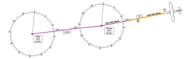
Figure 7-33 Transition to GPS Flight Plan
