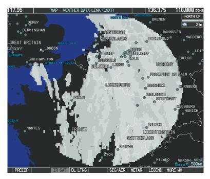
Figure 6-72 Infrared Satellite Data on the Weather Data Link (GFDS) Page
