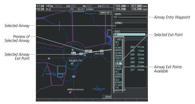
7) Press the **ENT** Key. The system returns to editing the flight plan with the new airway inserted.
