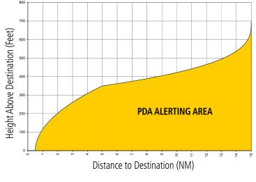
Figure 6-149 PDA Alerting Threshold
