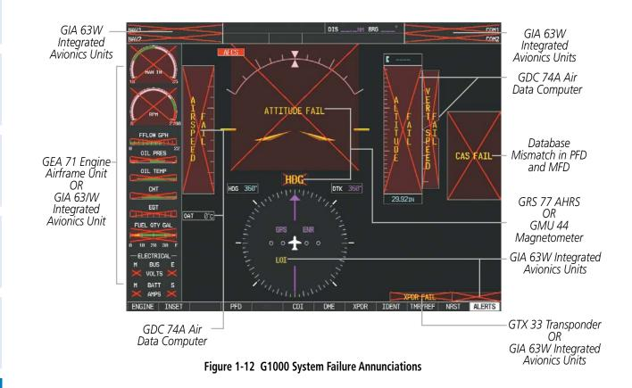
**NOTE:** Upon power-up, certain windows remain invalid as G1000 equipment begins to initialize. All windows should be operational within one minute of power-up. If any window continues to remain flagged, the G1000 System should be serviced by a Garmin-authorized repair facility.
