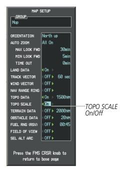
Figure 5-17 Navigation Map Setup Menu - TOPO SCALE Setup
