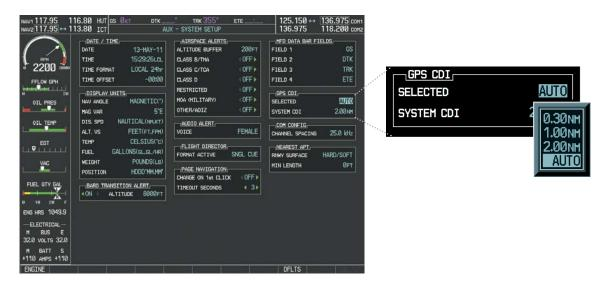
Figure 2-22 GPS CDI Settings (AUX - System Setup Page)
