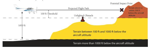
Figure 6-137 Terrain Altitude/Color Correlation for TAWS
