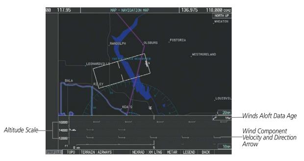
Figure 6-84 Navigation Map Page with Winds Aloft Data on Profile View
