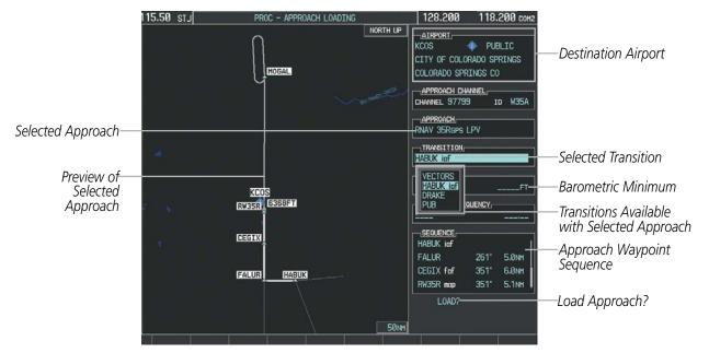
Figure 5-75 Approach Loading Page - Selecting the Transition
