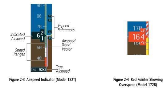
A color-coded (white, green, yellow, and red) speed range strip is located on the moving tape. The colors denote flaps operating range, normal operating range, caution range, and never-exceed speed ( $V_{_{NE}}$ ). A red range is also present for low speed awareness.
