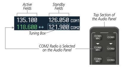
Figure 4-3 Selecting a COM Radio for Transmit
