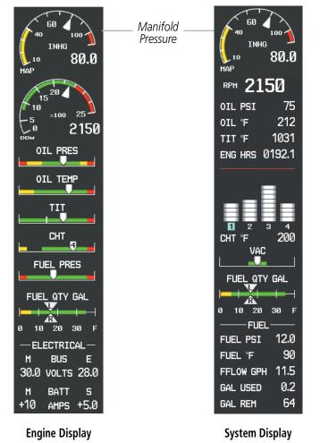
Figure 3-12 ECU Mechanical Backup Mode (Model J182T)
