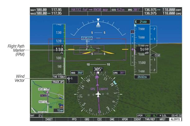
Figure 8-7 Flight Path Marker and Pathways
