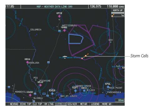
Figure 6-20 Cell Movement Data
