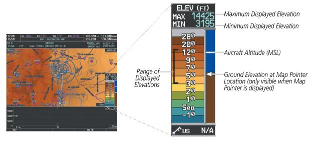
Figure 5-16 Navigation Map - TOPO SCALE
