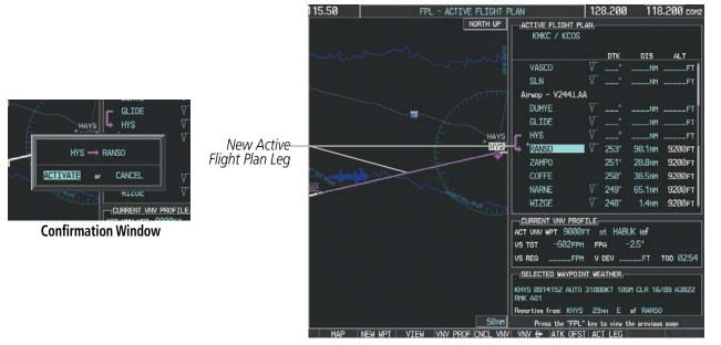
Figure 5-85 Active Flight Plan Page - New Active Leg
