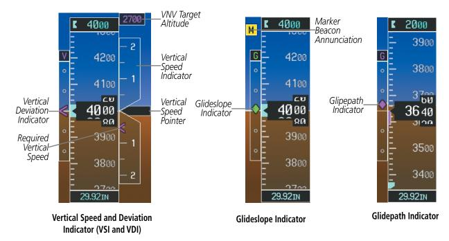
Figure 2-11 Vertical Speed and Vertical Deviation Indications
