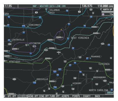
Figure 6-30 Freezing Level Weather Product
