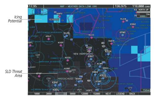
Figure 6-42 Icing Data at 6,000 Feet
