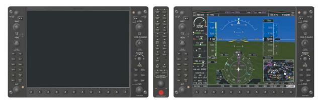
Figure 1-10 Reversionary Mode (Failed PFD)
