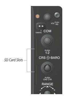
Figure 1-6 Display Bezel SD Card Slots
