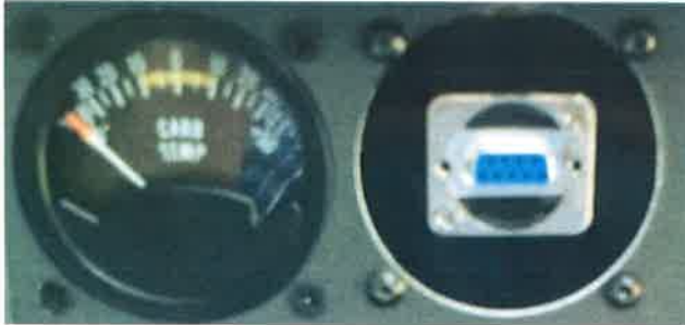
Figure 1.1.: Jack for OBU Logger mounted within metallic faceblade of an instrument slot
