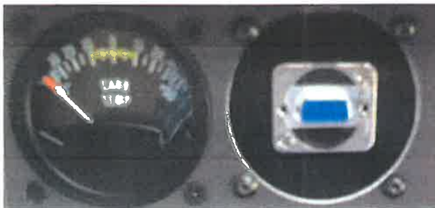
Figure 1.1.: Jack for OBU Logger mounted within metallic faceplate of an instrument slot
