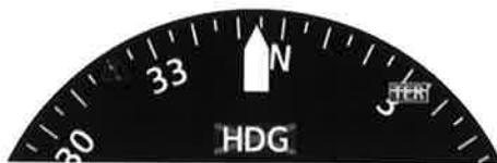
Figure 7- Top of the HSI when HDG failed (no GPS)
